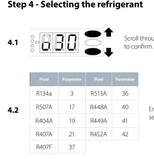
Scroll through parameters and select parameter o30, press the central button to confirm.
