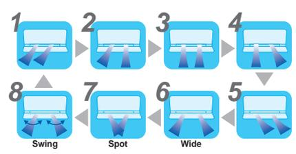
The airflow direction from the right and left louvers can be controlled individually. Eight different air flow patterns can be selected.
