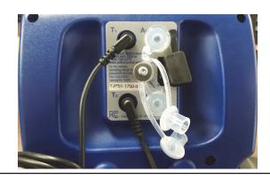
Plug the low side temperature probe into T1 on the back of the device. Plug the high side temperature probe into T2 on the back of the device.
